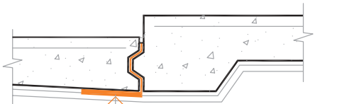
KORDON TB taped on top of DPM - option B
